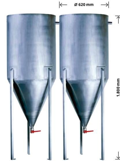
Sedimenter for cleaning through sedimentation. To be used individually or in together with a chamber filter press. Weight 54 kg, contents per sedimenter 270 litre
